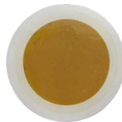
Critical varnish potential
